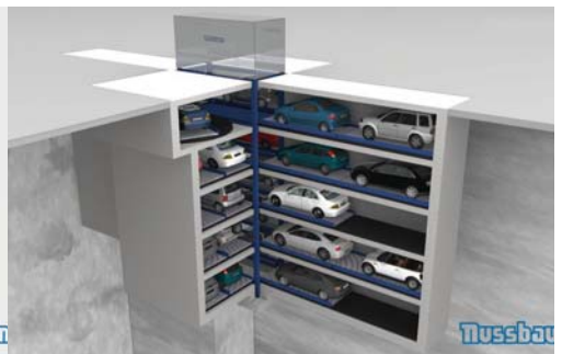
SMART PARKER MAX-XY (lengthwise and cross conveyor)
